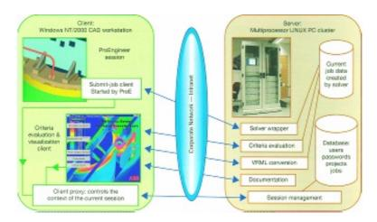
${\it Client-server \ architecture \ for \ accessing \ the \ remote \ resources \ integrated \ with \ CAD \ environment}$ and design criteria evaluation
